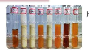
High concentration mixing without reaction and stratification
